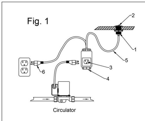
If there is no appropriate hole for mounting the Button Body, drill a 1-3/8" (35mm) diameter hole into your counter or sink in a location accessible to the user.
