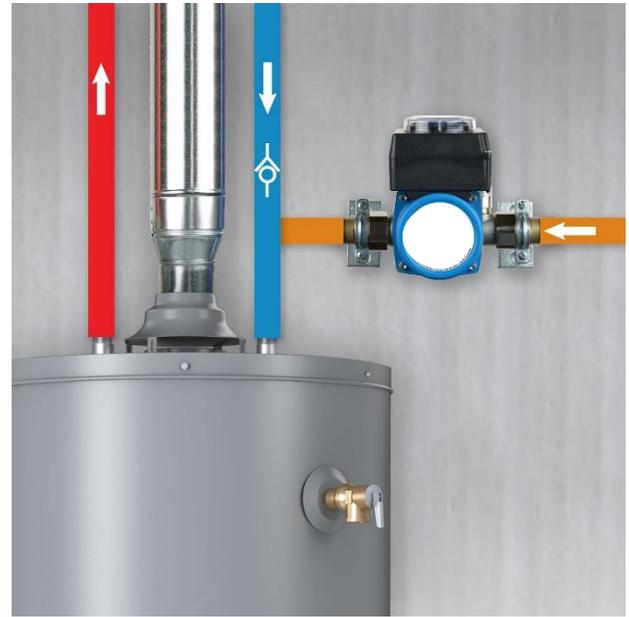
**Mount pump at least 3 Feet from the cold discharge from the tank. If a check valve is used in the cold water line, connect the dedicated return line to the cold water supply to the tank between the tank and the check valve.**
