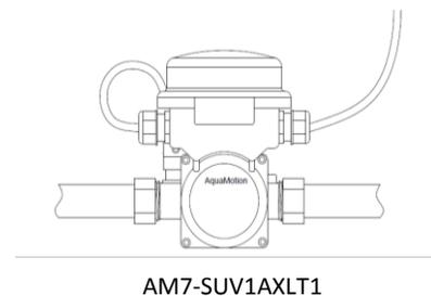
To protect the circulator from water intrusion the box, must always be mounted upwards as shown.
